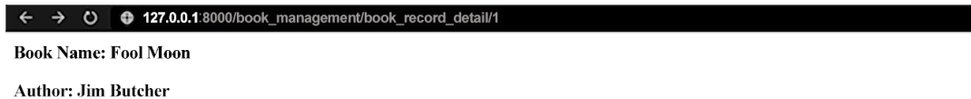
Figure 11.9: View rendered when we try to access a previously stored book record
